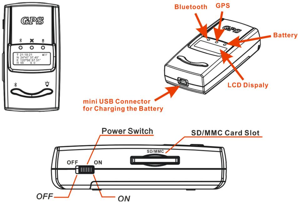
There are three LED windows on the front cover to indicate the GPS, Bluetooth and battery status. One LCD display panel on the front cover shows time, longitude, latitude, height, speed, battery status, SD/MMC Card, and satellite signal status. Detailed LED and LCD indications are described in next paragraph. The battery on/off switch and SD/MMC card slot are located on the same broadside of the body. The mini USB port for charging the battery is on the down side of the body.
