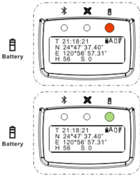
**Battery Low : Red LED Flashing**
